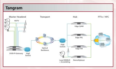
For IPTV contribution and end to end IPTV based video for residential customers in IP only networks like xPON, P2P, xDSL and DOCSIS based IPTV in HFC TANGRAM supports various encoding standards (MPEG2, MPEG4 received from satellite and terrestrial sources) and container formats (MPEG2-TS, MP4) as well as high density re-multiplexing, transrating and transcoding besides CBR and VBR processing.
