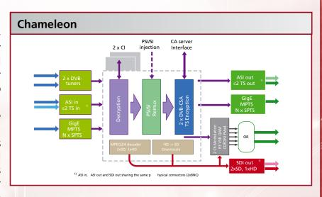
the internal tuners later as a local backup in case the IP source fails. Modules can work as an IP-Gateway (streamer) for DVB-S/S2/T/C signals to feed a backbone and at the same time produce 2 QAM outputs for the local network. Analogue Audio Video or digital baseband SDI signals can be encoded to MPEG2/4 and multiplexed into any DVB-C, DVB-T,IP or ASI stream. When analogue input becomes obsolete you can activate the module as transcoder for MPEG4 to MPEG2.
