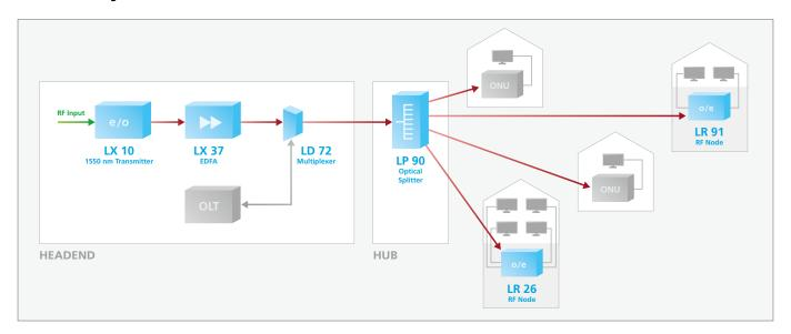
Offering broadcast TV services in todays FTTx networks is easily realized using 1550 nm transmitters together with high power EDFAs. The Optopus product family includes external modulated
