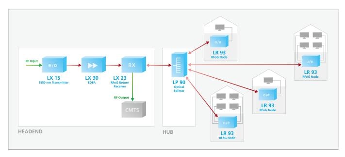
Optopus includes the components for RF over Glass networks, the cable operators' choice for FTTx applications. Depending on the size of network and distances to cover, Optopus offers a range of external or direct modulated transmitters and high power EDFAs. The RF over Glass receiver LX 23 with its very low noise receivers ensures optimization of the network even in challenging topologies.
