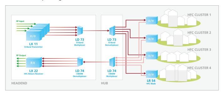
Optopus includes the full range of transmitters, return receivers and optical passives for every HFC application. Also, using O-Band WDM technology with the fullband transmitters LX 11 it is possible to reduce HFC cluster sizes without deployment of additional fiber, reducing the cost of a bandwidth increase significantly.
