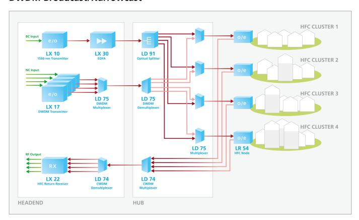
State-of-the-art broadcast/narrowcast applications using DWDM transmission for the narrowcast are a strength of Optopus. Broadcast services are transmitted over long distance links using external modulated transmitters LX 10,
